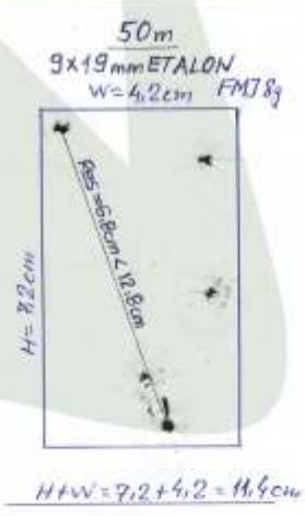
Picture of simultaneous shots on 25m and 50m for 9x19mm FMJ, 8g
