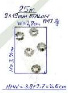
Picture of simultaneous shots on 25m and 50m for 9x19mm FMJ, 8g
