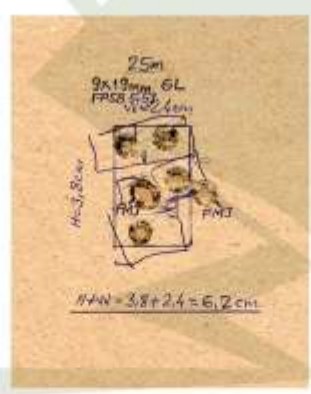
Picture of simultaneous shots on 25m and 50m for Sinter bullet 9x19mm FPSB, 5,5g and two bullets 9x19mm FMJ, 8g
